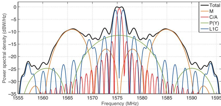
**FIGURE 1** Theoretical spectra of the four signals transmitted by a GPS III satellite in the L1 frequency band.
